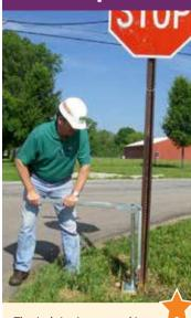
The Jack Jaw's patented jaw mechanism provides a positive grip that prevents strain and gives you a 16:1 mechanical advantage. The Jack Jaw 500 series super pullers, also available.
